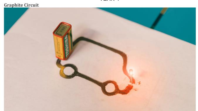
Can you complete an LED circuit using a normal graphite pencil? Learn about the conductive properties of graphite and draw your own design to see it light up!
