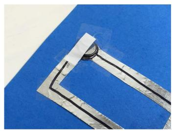
Cut a small piece of rectangular foil with paper backing (from step 5).
