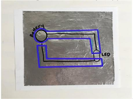
Draw out a circuit with a coloured sharpie. In our example, we used a blue marker to draw our circuit. Cut out a piece of foil to practice drawing a circuit!
