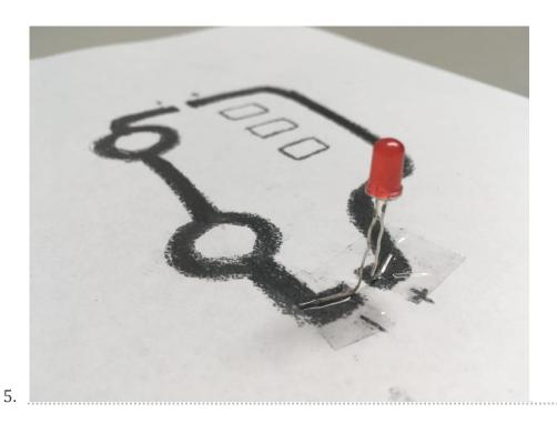
Tape the wire at the end of the lines across the other gap, aligning positive and negative wires. Make sure your LED stands upright. The wires should be in contact with the graphite lines.
