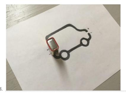
Once you're done with your design, place the battery on one of the gaps. Align the positive and negative ends with the graphite lines.
