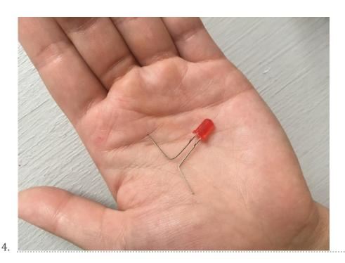
Take an LED and bend the bottom ends of the wires.
