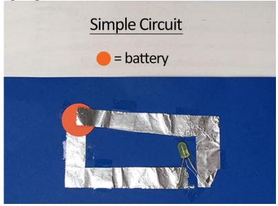
Note: In this step we used regular LEDs (they have the two wires!), and sewable LEDs (looks like an oval!). Any kind of LEDs work - just be sure the LED, as well as the battery have good contact with the foil and that there is no tape in between the parts and the foil.
