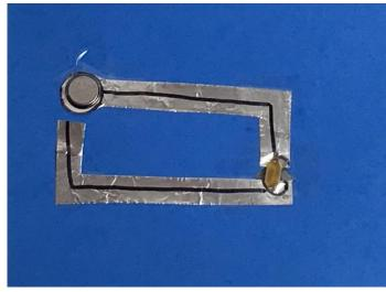
Cut out the foil paths by following the coloured lines. Use clear tape to tape the foil paths to the back of your card.
